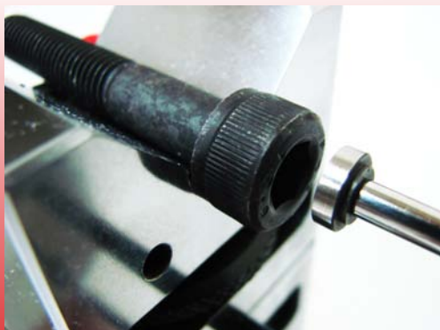
Screw head thickness measuring
