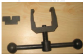
Device to dismantle pendulum
