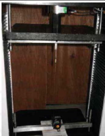
Ring stiffness pipe inner deformation measuring device
